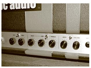
The Body control changes the low and low-mid frequency response of the amp. Very versatile and useful, particularly when driving the amp harder.
